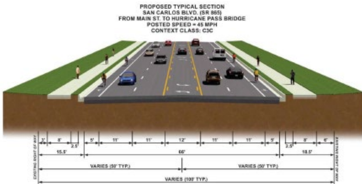
Figure 3. Typical Section of the SR 865 (San Carlos Blvd.) improvements from Main Street north to Hurricane Pass Bridge
