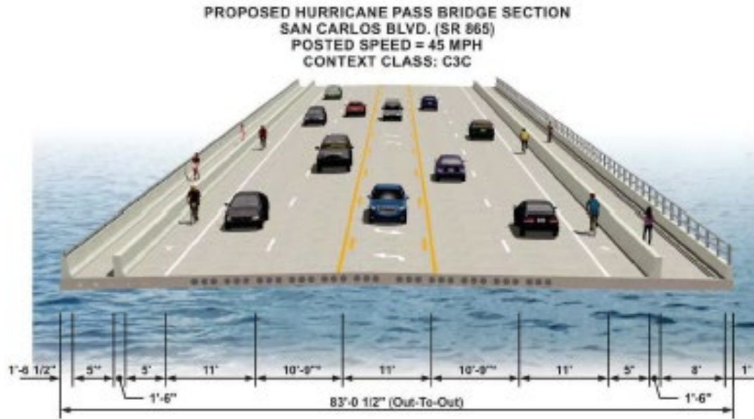
Figure 4. Typical Section of the proposed Hurricane Pass Bridge improvements
