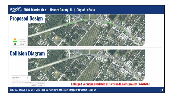
The proposed design plans are available for review on the project website. They have been placed above a map summarizing the collisions identified in the 2024 Access Management Study to compare crash locations and the placement of the proposed median.
