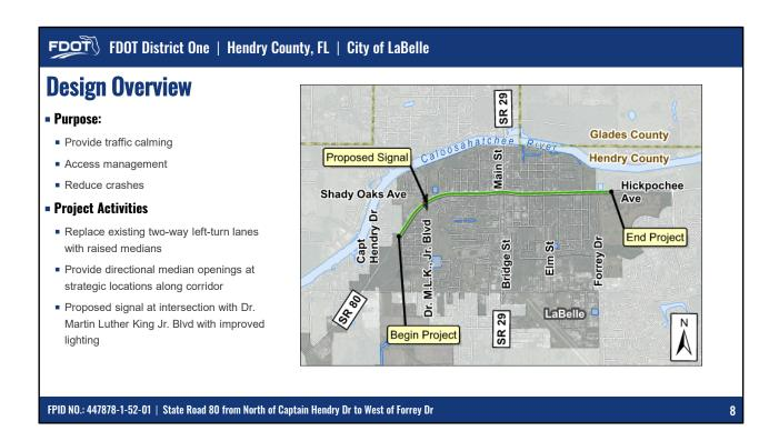
The proposed design plans include intersection reconfigurations, the addition of raised medians to the existing two-way left-turn lanes, and a new traffic signal at the intersection of Dr. Martin Luther King Blvd. Additional project elements include addressing any needed structural or drainage deficiencies. All project elements are anticipated to occur within the existing public right-of-way.
