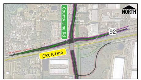
**ALTERNATIVE 1 -** This is an elevated intersection. Elevating both County Line Road and US 92. County Line Road goes over CSX A-Line.
