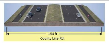
County Line Road proposed six-lane typical section consists of three-lanes in each direction (36 ft wide) separated by a 30 ft median with 10 ft shared use paths on both sides.
