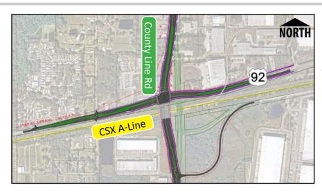
**ALTERNATIVE 1 -** This is an elevated intersection. Elevating both County Line Road and US 92. County Line Road goes over CSX A-Line.
