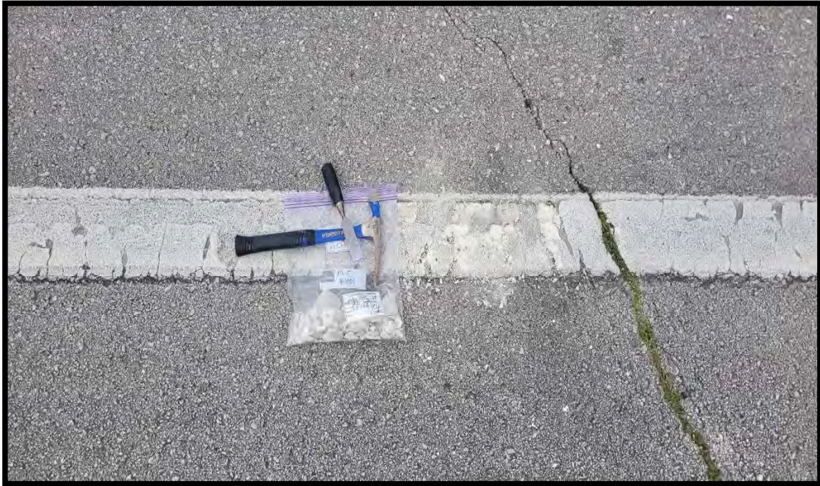
Photograph 91 View of Metal Based Coatings Sample PS-5 White Lane Paint – Bridge 910002.
