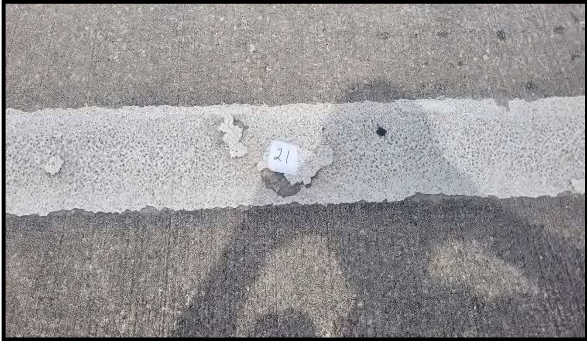
Photograph 23 View of Asbestos Homogeneous Area 7 – White Lane Paint – White Striping of Bridge 910001 (Sample Location 21).
