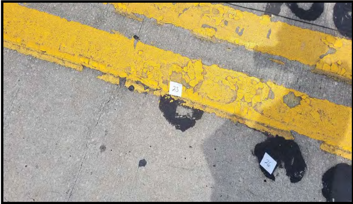
Photograph 25 View of Asbestos Homogeneous Area 8 – Yellow Lane Paint – Yellow Striping of Bridge 910001 (Sample Location 23).
