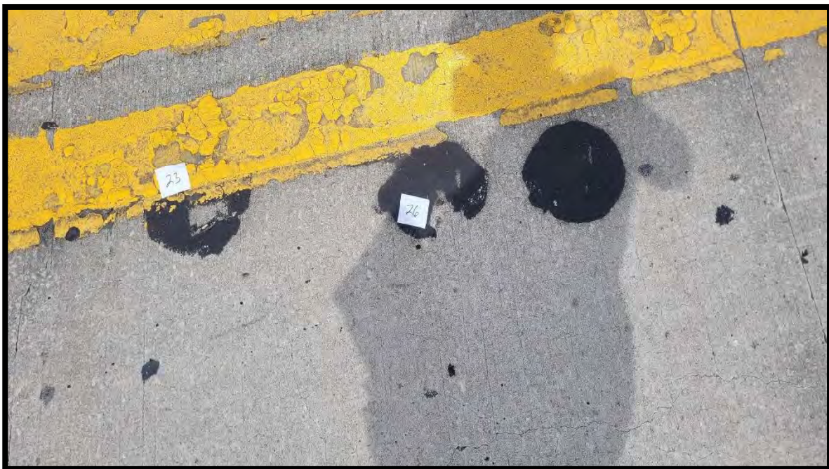
Photograph 28 View of Asbestos Homogeneous Area 9 – Black Adhesive – Surface Reflectors of Bridge 910001 (Sample Location 26).
