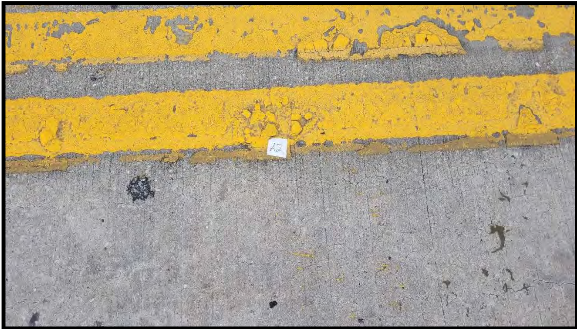
Photograph 24 View of Asbestos Homogeneous Area 8 – Yellow Lane Paint – Yellow Striping of Bridge 910001 (Sample Location 22).
