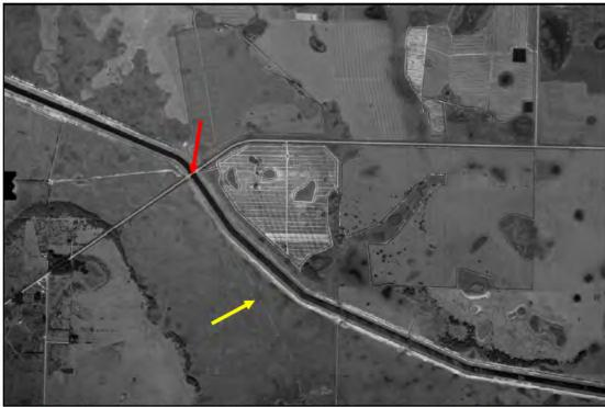
**Figure 5.10.** 1970 aerial photograph depicting the newly constructed Slough Ditch Canal (C-41A) (FDOT 1970). The bridge carrying SR 70 (APE) over the waterway is indicated by the red arrow. The extant original alignment of Slough Ditch is indicated by the yellow arrow.
