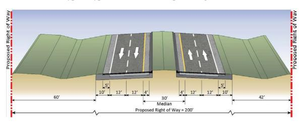
Figure 1.8 SR 29 Bypass Typical Section from Gopher Ridge Road to SR 29
