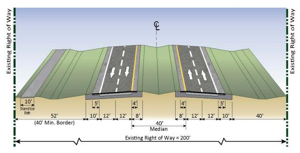
Figure 1.6 SR 29 Typical Section from Experimental Road to South of SR 82
