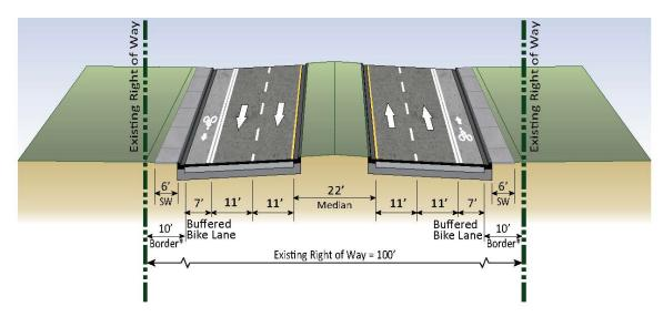
Figure 1.3 SR 29 Typical Section from North of Seminole Crossing Trail to CR 846
