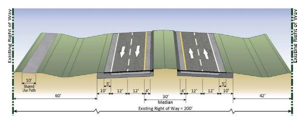
Figure 1.5 SR 29 Typical Section from the SR 29 Bypass Junction to Experimental Road
