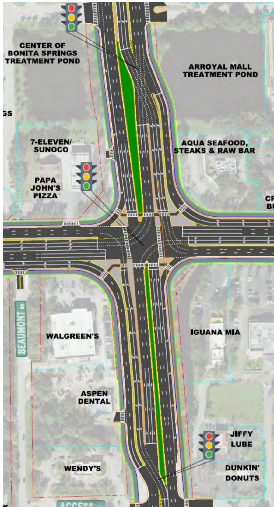
Figure 1.3. Alternative B – Partial Displaced Left Turn.
