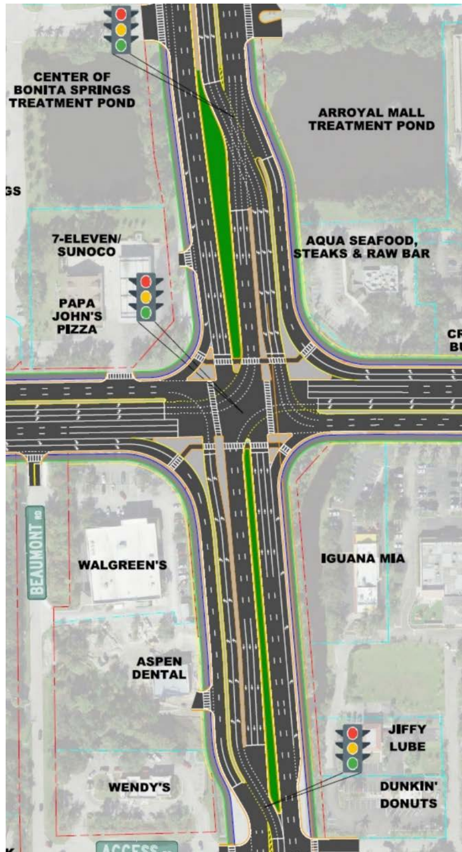
Figure 7: Alternative B – Partial Displaced Left Turn
