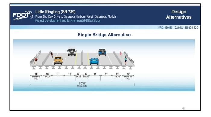
The single bridge alternative will replace the two existing bridges with a single structure for all lanes of travel. The travel lanes on the new bridge will be the same 11-foot width as on the existing bridges. 10-foot outside shoulders will accommodate bicyclists, and a 14' shared use path would be added to each side of the bridge.
