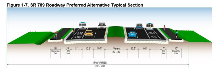
Design variations for lane width and bridge shoulder (median and outside shoulders) widths will be required for the Preferred Alternative.
