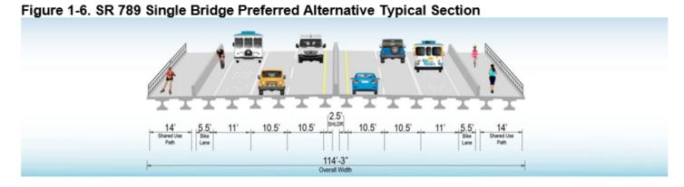
The new bridge will transition to a curb and gutter roadway typical section that includes two 10.5-ft wide travel lanes, a dedicated 11-ft bus on shoulder, and 5-ft bike lane in each direction, separated by a median with Type E curb and gutter. This section of roadway also includes a 10-ft shared-use path on both sides of the roadway that connects to the bridge, shown in Figure 1-7. No ROW will be required. The design speed is 40 mph with a posted and target speed of 35 mph.
