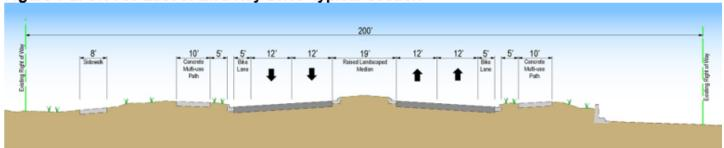
From Bird Key Drive to the existing bridges, the existing typical section includes two 12-foot-wide travel lanes in each direction, separated by a curb and gutter and flush landscaped median ranging in width from a minimum of 12 feet to a maximum of 76 feet. This section of roadway also includes 4-ft wide paved shoulders and a 10-ft multi-use path on the north side and a meandering 10-ft multi-use path within Bird Key Park that connects to the existing bridges, shown in **Figure 1-3**.
