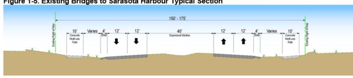
Figure 1-5. Existing Bridges to Sarasota Harbour Typical Section
